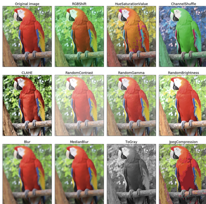
Figure 2.2: Example of data augmentation through colour and blur variations from the Albumentations library. Data augmentation is a widely used technique for generating synthetic data. [2]
