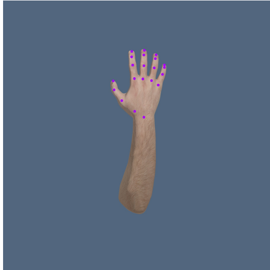
Figure 4.2: View of the baseline configuration of the synthetic dataset generator, showing the procedural hand model in an idle position. The purple circles represent the projected keypoints.
